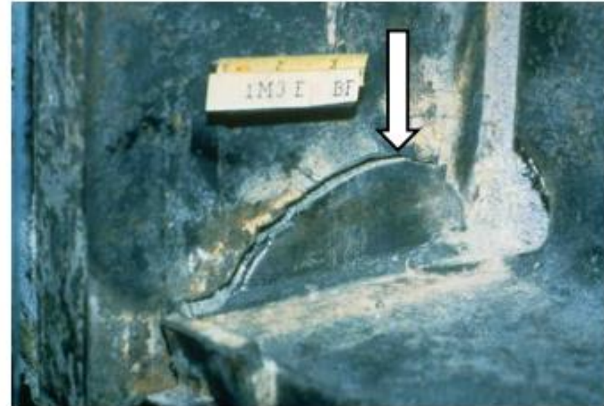
Fig. 6-3. Fracture involving divot of steel being withdrawn from column flange. (Photo by Dave Norris)
